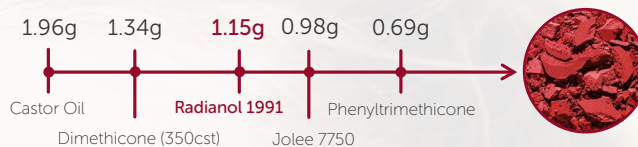
Graph 1: Amount of emollient (gram) needed to solubilize 1 gram of pigments. Ref Isoamyl laurate / Jolee 7750 = 0.98g. Pigment : Iron oxides CI77491 Jojoba esters (coated)
